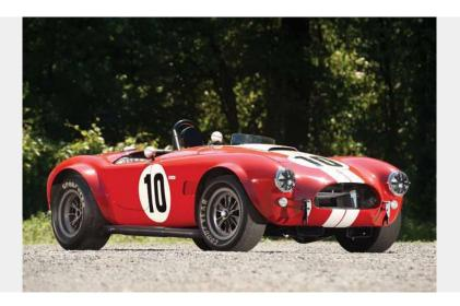
Keen to show well in auto test competition, Shelby came up with the Slalom Snake to show the Cobra was about more than just **straight-line** speed. To improve the handling, the two Slalom cars built had Koni shock absorbers, front and rear anti-roll bars fitted, and **Goodyear** Blue Streak Sports Car Special tyres.
