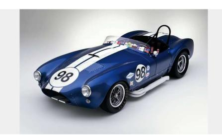
The 390 Big Block was the first **dabble** with larger engines for the Cobra. However, this 390ci (6.4-liter) motor was no normal V8. It was an all-aluminium engine borrowed from Ford's **NASCAR** program and had **flip-open** bodywork to make it easier to get at the mechanical components front and back. This earned it the nickname 'Flip-Top'.
